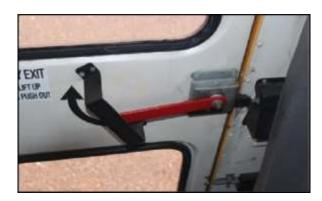
To open the emergency exit, a person must unlatch the door by pulling the red lever upward, and then push against the door.
